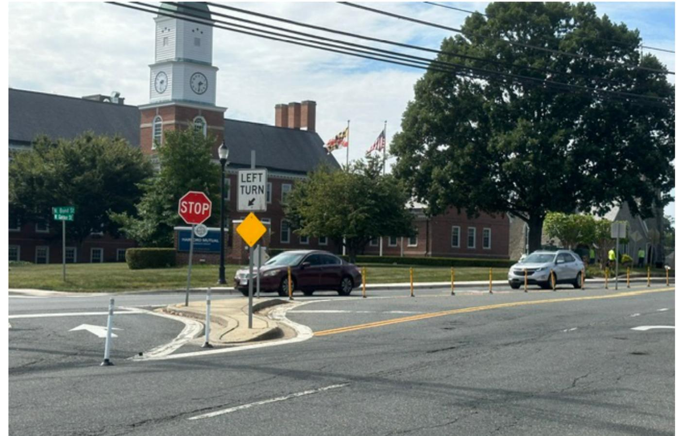
Flex posts are used to close the left turn onto E Gordon St, which simplifies the intersection (Source: Laura Bianca-Pruett, Town of Bel Air)
